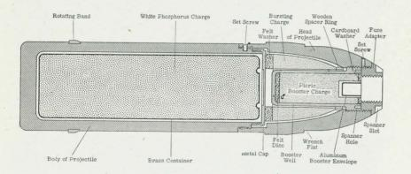
in diameter, and containing a well for the aluminum booster envelope. A felt disk is glued to the bottom of the cylinder.
