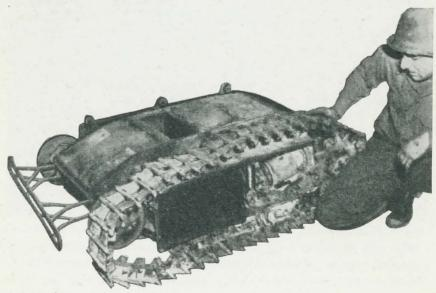
A DAMAGED GOLIATH, LINE-CONTROLLED DEMOLITION VEHICLE.
