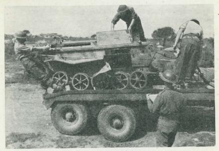
THE B-4 RADIO-CONTROLLED DEMOLITION VEHICLE.
