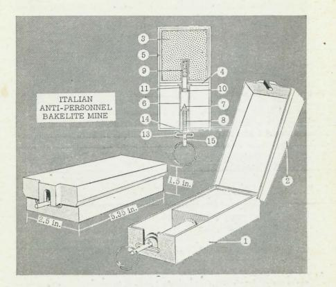
To neutralize the mine, carefully lift the lid clear of the actuating pin (13). Place a wire in inner hole (15) and lift out the whole striker assembly. Unscrew the locking ring (11) and take out the detonator.
